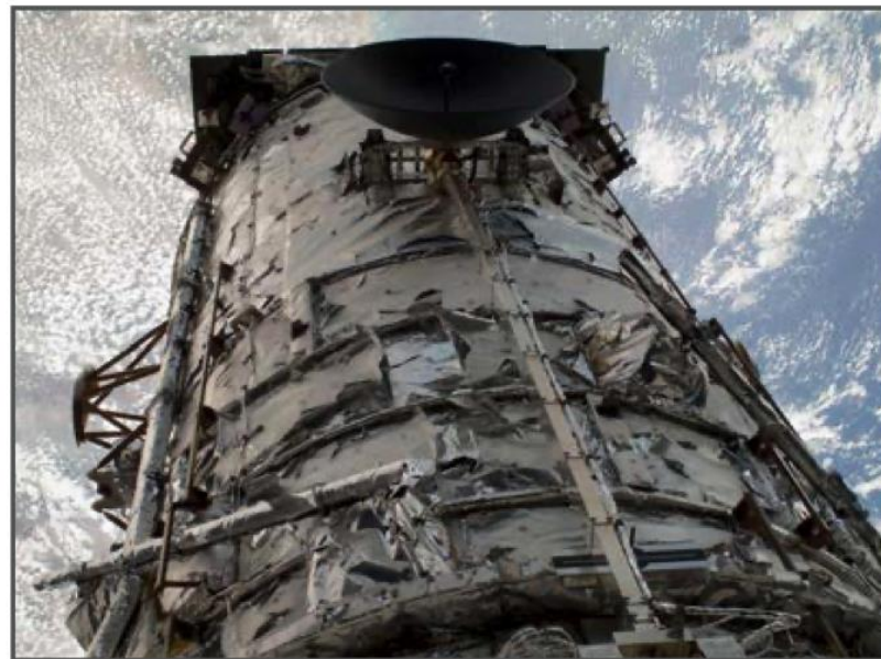
Severe degradation to the aluminized-Teflon ® outer layer of multilayer insulation after 19 years of space exposure (Yang and de Groh, 2010).
